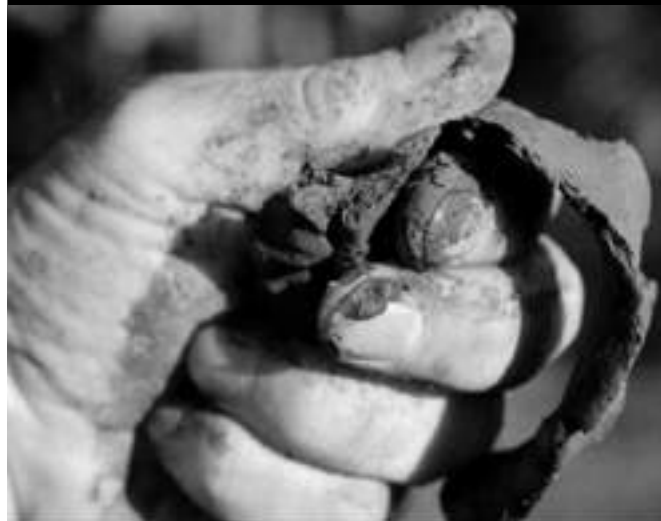
Figure 1: Making a soil ribbon
